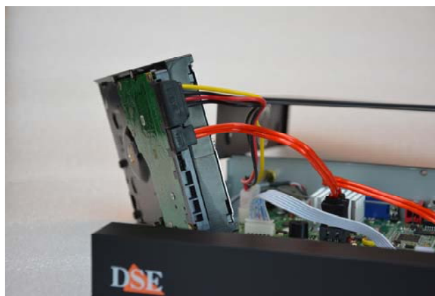
Connect the hard drive with two power and data cables that are inside
