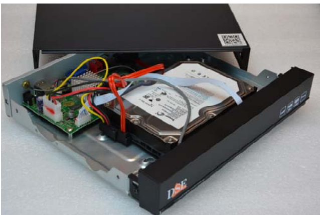
Fix the hard disk with 4 screws which are screwed are screwed from underneath the VCR
