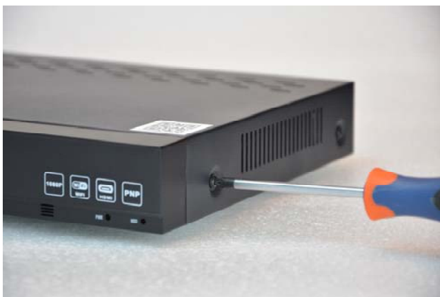
Remove the cover by unscrewing the 5 screws: 2 on each side and a rear
